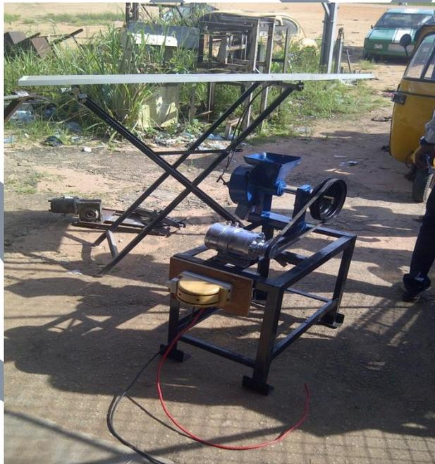
**Fig. 1. Fabricated grain grinding machine.**
